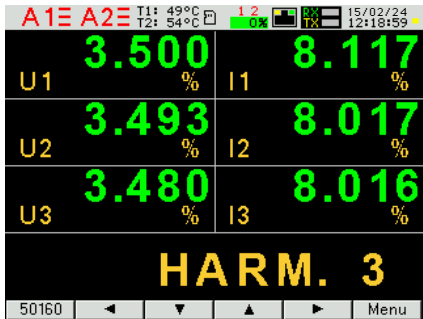
Fig. 19. Screens 11 and 12 - visualization of harmonics
