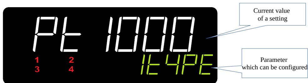
Fig. 8: View of menu when setting a parameter.
